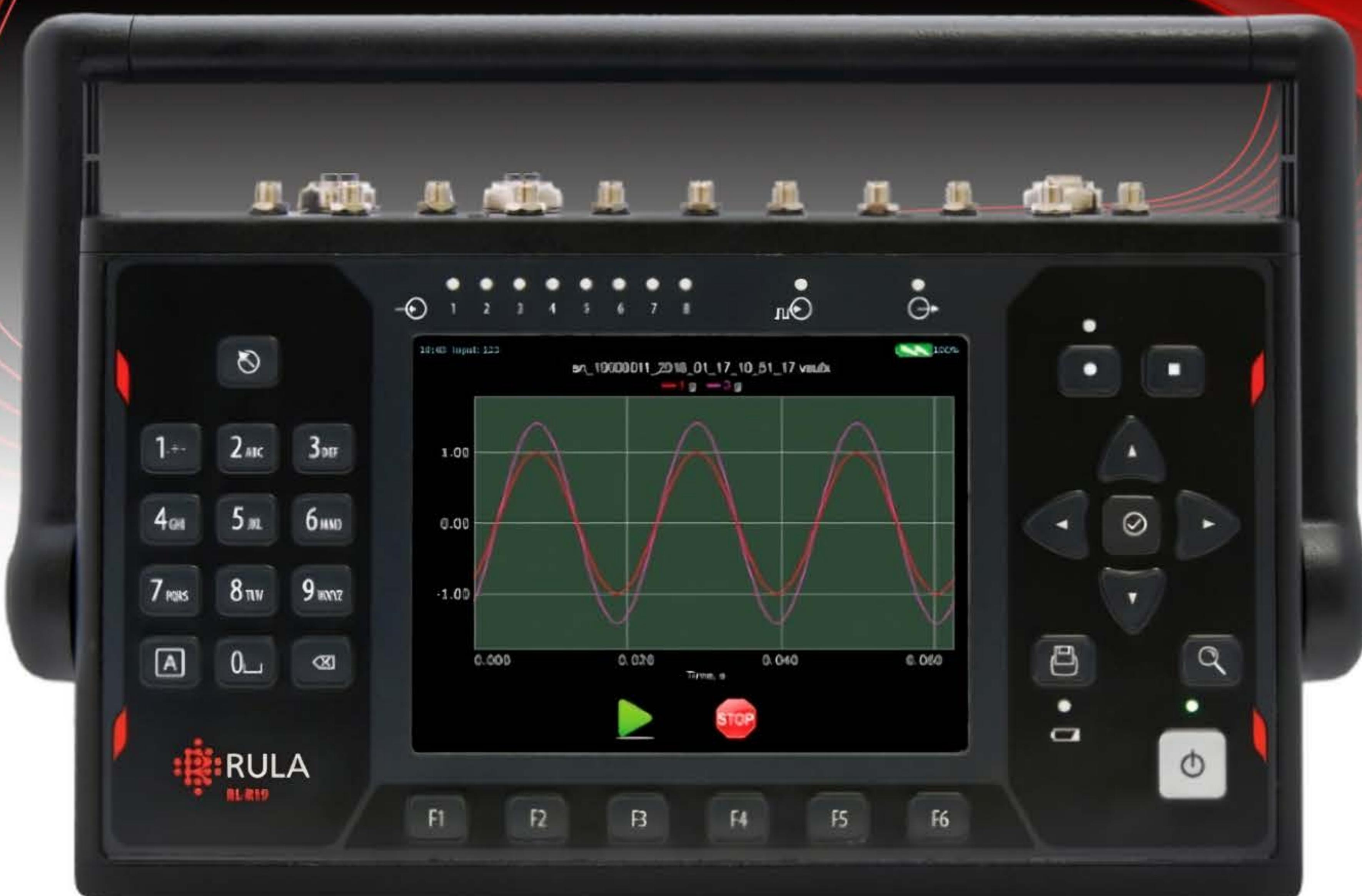
RL-R19 DAQ system and spectrum analyzer is intended for measuring and recording vibration data and other physical processes. RL-R19 enables the user to:
