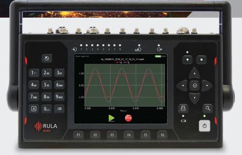
RL-R19 DAQ system and spectrum analyzer is intended for measuring, registering and analyzing vibration data and other physical processes. RL-R19 enables the user to:
